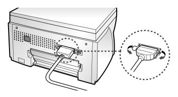
Plug the other end of the cable into the appropriate parallel 4 connector on your computer and fasten it tight.
